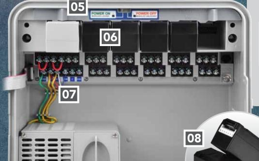
O5 Sliding the Power Lock turns the controller's power on or off. This permits the addition or removal of output modules and locks the modules into place in the power on position.
